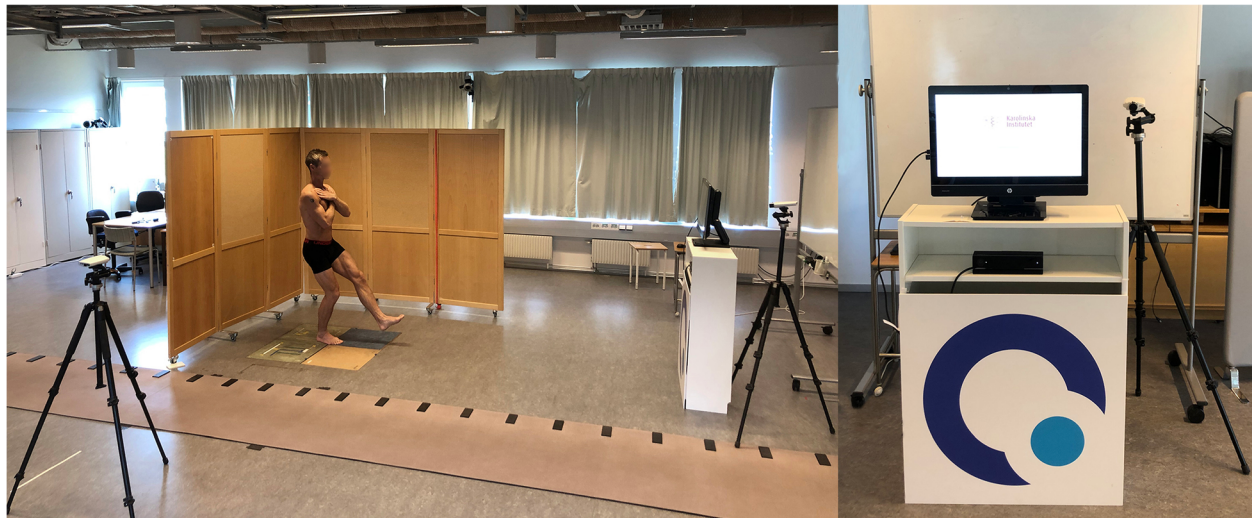
Fig. 1 The set-up of Qinematic™ during the data collection of the Single Leg Squat. The two orthogonally placed cameras are shown in the figures, right figure shows the subjects view in front of the Kinect camera and computer touchscreen
